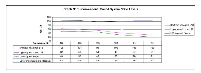
This test established a noise limit for the dance floor of 103 dB(C) at 3m from the sound system speakers.
