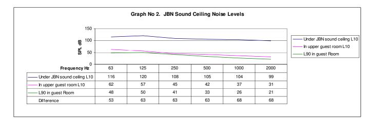
These tests resulted in an allowable noise level on the dance floor of 113 dB(C), ie an increase in allowable amplified entertainment of 10 dB over the original installed conventional sound system.
